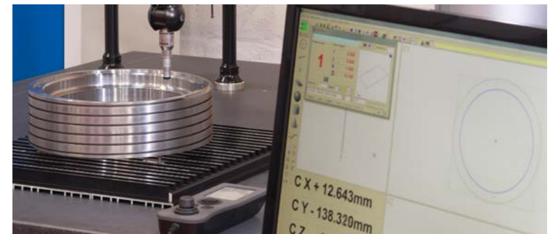
Coordinate-measuring machines are used to guarantee absolute precision in the slip ring production
