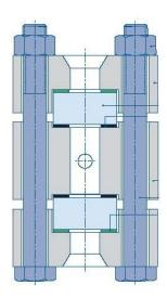
Two transparent glasses are clamped into the display body and close off the liquid channel to the front and rear. If necessary, an illumination device can be attached to the rear of the display body.
