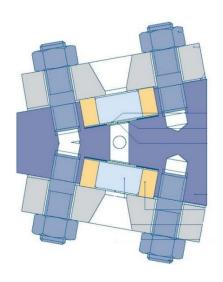
In principle, a transparent indicator, but with wedge-shaped center piece. This enables the two-color display: in the illumination display there are two color filters - one red and one green.
