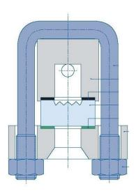
The principle is based on the displacement of the refractive index of liquid and gas or water and steam. The liquid column is located in the trough of the centerpiece behind the sight glass, which is clamped in the indicator body.
