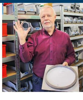
rings was removed and "we were able to pinpoint the problem to the installation density of the graphite rings, which was much too low."
