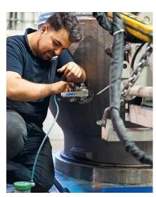
A bubble counter is mounted on the valve cavity to verify tightness in accordance with EN 12266-1 P12.
